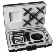
The multifunction model ADM-870C provides digital display of readings in English and metric units corrected for **local or standard** density. Features include **auto-read**, memory with total and average, display of **associated** pressure and temperature, VelGrid, AirFoil probe and **serial output to printer or computer**. Measures air velocity, absolute and differential pressure, temperature, and backpressure compensated air flow when used with the series 8400 FlowHood.
